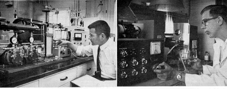
DYNAMIC SOLVENT vapor generator is being used by D. R. Parker (3311) to calibrate a halide meter for accurate readings in the field. The generator produces standard concentrations of gases or vapor which can check the accuracy of air sampling equipment used by industrial hygienist.
